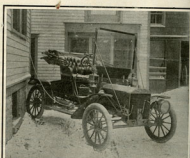
The Gas Generator on the Automobile Was Connected With the Lamp by a Piece of Rubber Drainage Tubing.
