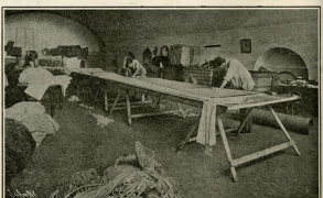
In an English Balloon Factory. Cutting the Cloth Into Properly Shaped Segments. HOW TO CONSTRUCT A BALLOON.
