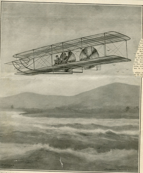
This Aeroplane is the First Dynamic Flying Machine to Traverse a Considerable Distance and Carry Two Men at a Speed of 45 Miles an Hour. A Similar Aeroplane to be Built for the United States Government by the Late August Next Remains in the Air for an Hour and Cover 40 Miles in That Time.
