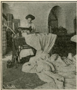
Setting Together Segments of Cloth Into Balloon Cases.
